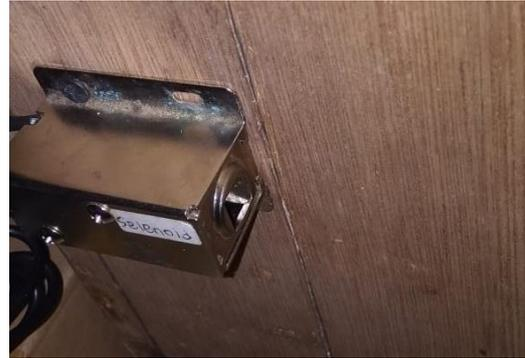
Gambar 12. Open solenoid Door Lock 1
