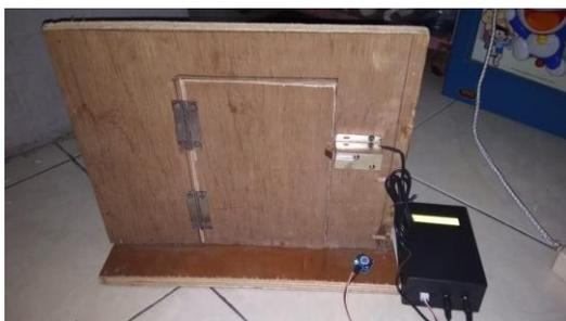
Gambar 7. Pintu Solenoid Door Lock
