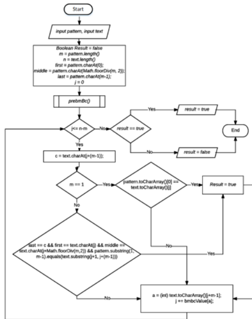
Gambar 4. Flowchart Algoritma Raita
