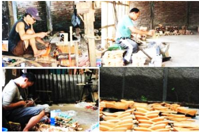
Figure 5 The activities of craftsmen when the process of the formation of Clogs (Source: Asep Sufyan Documentation, 2015)
