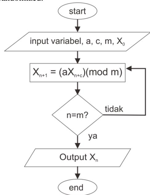
**Figure 2.** Flowchart Algoritma LCM
