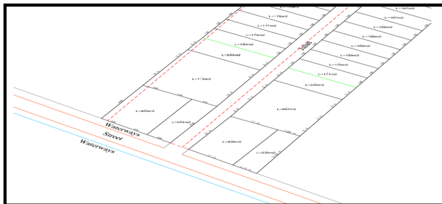
Figure 2. Example of Ground Splitting Process for Housing
